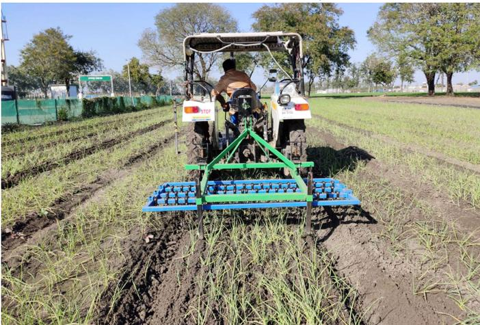
Weeds are the major problem for low productivity of garlic which compete with garlic crop for soil nutrients. A tractor drawn garlic weeder has been developed for weeding in garlic crop sown on broad beds. The row- to- row spacing of the developed unit can be adjusted from 100 to 150 mm. The effective field capacity and weeding
