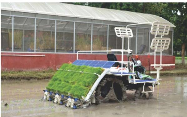
developed remote-controlled system on commercial rice transplanter has good control in the puddled paddy field. The field capacity, field efficiency and fuel consumption of the developed remote-controlled ride-on-rice transplanter have been 0.24 ha/h, 71% and 3.1 l/ha, respectively at forward speed of 1.61 km/h at slip rate of 12%.
